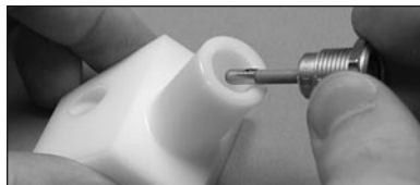
Figure 8 Insert replacement LEMO assembly
