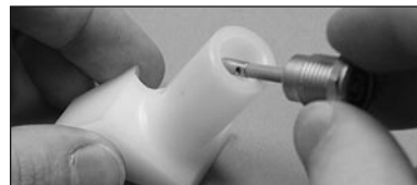
Figure 6 Insert replacement LEMO assembly
