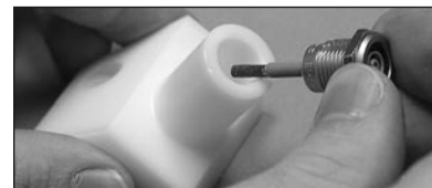
Figure 6 Remove LEMO connector
