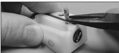
Figure 4 Screw spring bellows replacement assembly into CTM base
