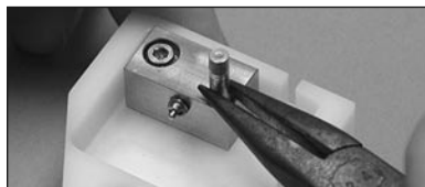
Figure 5 Screw spring bellows into block
