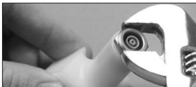
Figure 5 Remove the high-voltage LEMO connector
