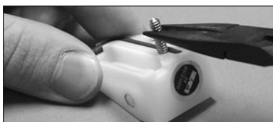
Figure 2 Loosen set screw with pliers and remove
