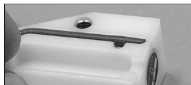
Figure 3 Set screw removed
