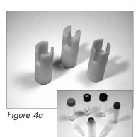
2. Three inserts (Figure 4a) are available to hold a wide variety of sample vials (Figure 4b). They are located in the accessories box. Choose the most appropriate insert for your sample vial and place both in the pressure vessel as shown in Figure 5. The pressure vessel features a spring-loaded well to allow the insert to be easily inserted and removed.
