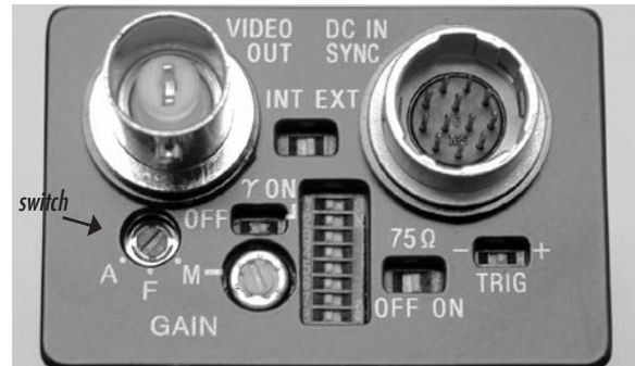
Figure 4.2: CCD camera gain switch set to automatic
