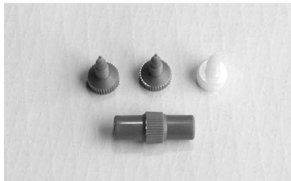
Figure 5.2: MicroTight® union, gauge plug, and compression fittings
