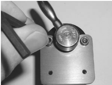
Figure 7.1: Upchurch valves require the included backplate be attached prior to mounting
