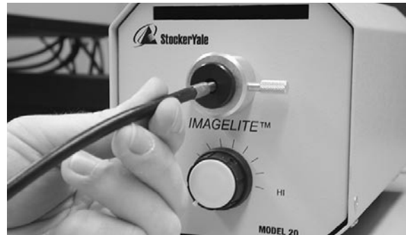
Figure 4.10: Install fiber optic bundle
