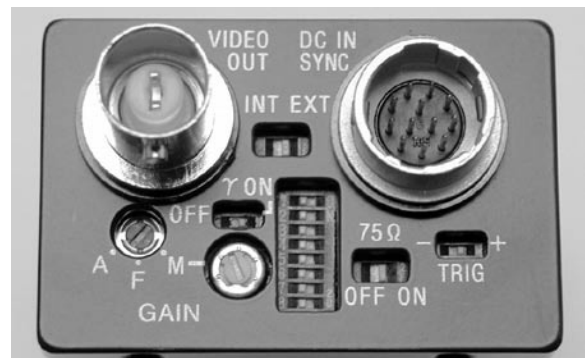
Figure 4.2: CCD camera gain switch set to automatic
