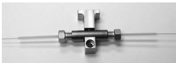
Figure 5.26: Fully assembled ZDV union
