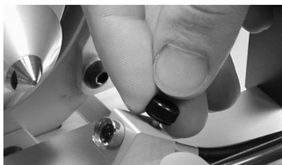
Figure 4.6: When locking the fiber optic bundle in place, do not overtighten thumb screw
