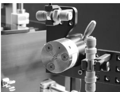
Figure 7.6: Component clamps with injection adapter and an IntegraFrit™ trap column
