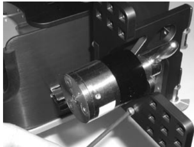
Figure 7.2: Attach the backplate to the mount using two mounting screws
