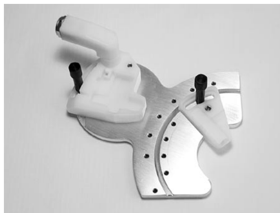
Figure 5.15: UTM and tip holder bases attached to stage plate
