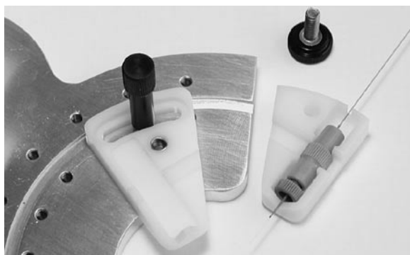
Figure 5.18: Union installed in the tip holder
