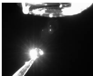
Figure 6.1: 850V Drops stick to tip
