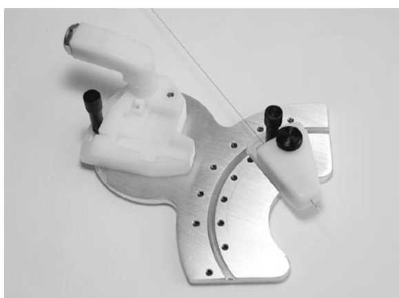
Figure 5.19: Union installed in the tip holder
