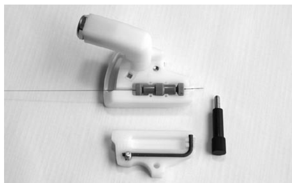
Figure 5.8: MicroTight® union inserted in the CTM base
