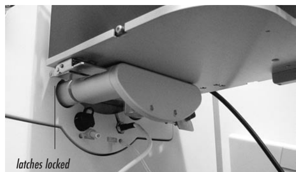
Figure 4.10: Latches locked firmly into place
