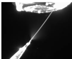
Figure 6.3: 1150V Droplet stream and spray
