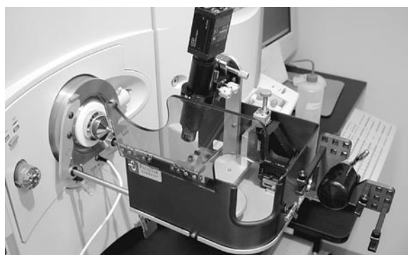
Figure 4.5 PicoView mounted on probe slide adapter
