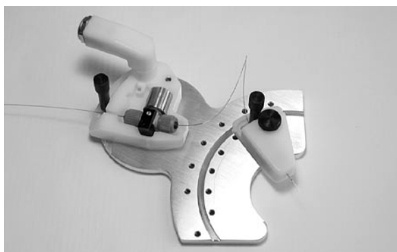
Figure 5.27: Plumbed MicroTee loaded in the UTM
