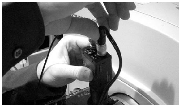
Figure 4.11: Connect the power cable to the camera
