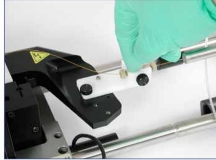
Plumb your PicoFrit Column into the PEEK union (refer to Making Connections). Place the PEEK union with loaded PicoFrit Column in the tip holder
