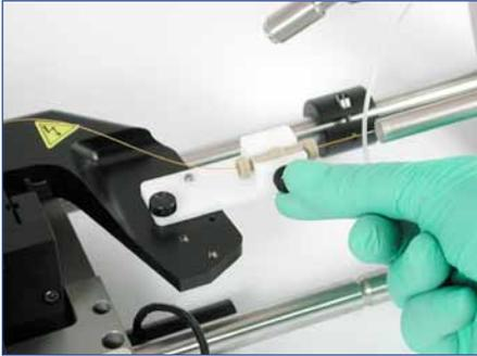
Tighten the locking screw to secure the union in place
