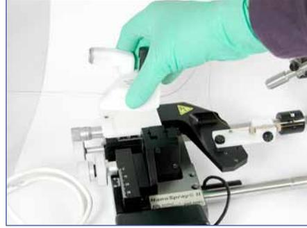
Place the UTM on the base. Measure, trim, and plumb the inlet end of the PicoFrit Column into the microtee along with the transfer line (refer to Making Connections for plumbing the tee).
