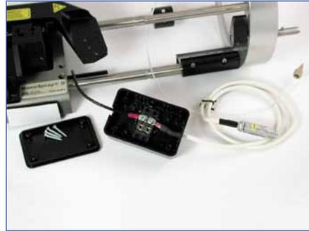
*Attach power lead from the Nanospray II source to the empty terminals in the power adapter. Tighten terminal screws (ADPC-NS2-4 only).*
