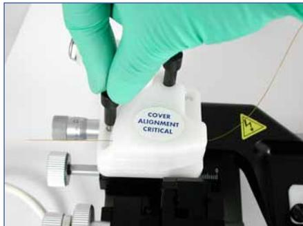
Insert the plumbed microtee into the UTM and affix the lid using a long thumbscrew. Attach the UTM to the base using the second long thumbscrew.
