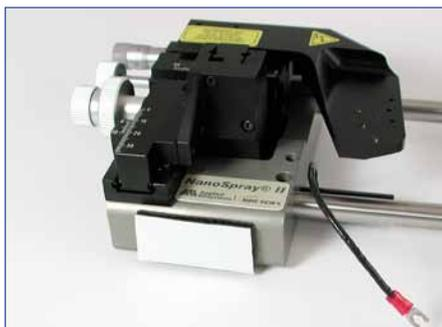
Attach Velcro tab to front face of the Nanospray II source base (ADPC-NS2-4 only)
