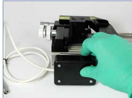
*Remove paper from Velcro tab; attach power adapter box to Velcro tab (ADPC-NS2-4 only)*
