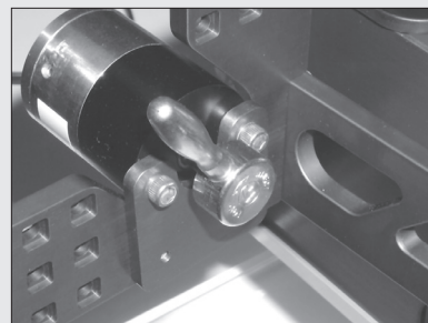
Figure 7.3 Properly mounted Upchurch valve
