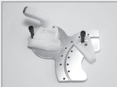
Figure 5.16 UTM and tip holder bases attached to stage plate
