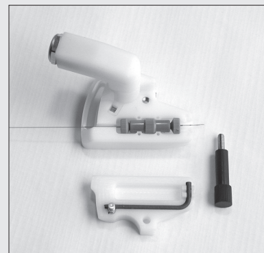
Figure 5.10 MicroTight® union inserted in the CTM base
