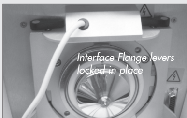
Figure 4.5 LTQ™ Interface Flange locked on the LTQ
