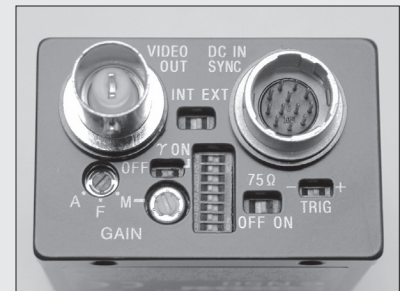
Figure 4.2 CCD camera gain switch set to automatic
