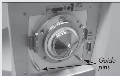
Figure 4.3 Attach brackets to source mounting flange
