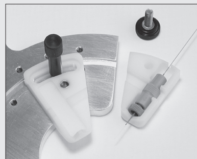
Figure 5.19 Union installed in the tip holder
