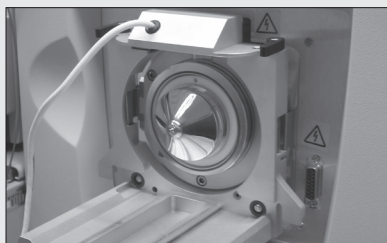
Figure 4.4 LTQ™ Interface Flange mounted on the LTQ
