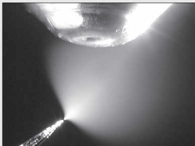
Figure 3.4 MS inlet and spray as seen through PicoView imaging system
