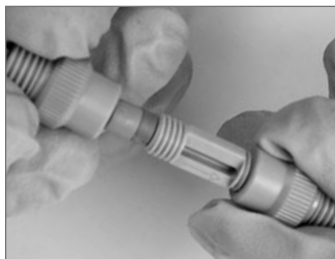
FIGURE 7 Set the nanofilter on the outlet end of the column holder assembly. Cover with the second end cap.
