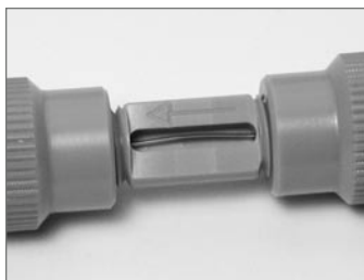
FIGURE 10 A slight bend in the installed column indicates a successful seal
