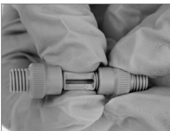
FIGURE 9 Gripping the column holder, securely tighten the end cap on the outlet end of the assembly
