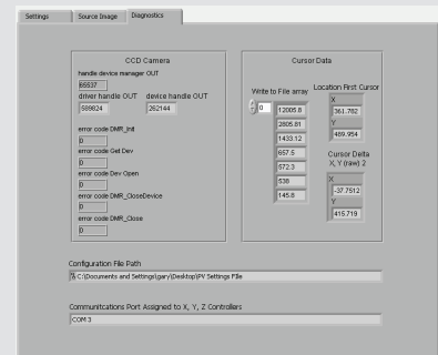
Figure 10.2 Diagnostics tab showing all camera connections are stable
